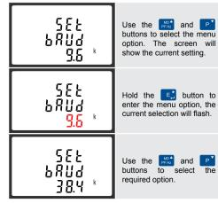
On completion of the entry procedure, hold the E button to confirm the setting
