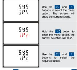
Hold the **E** button to confirm your adjustment. Hold the **W**
