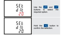
Hold the  $\mathbf{W}^{\mathbf{A}}$  button for 3 seconds to exit the set up menu.
