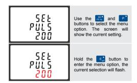
Use the wat and P buttons to choose the desired pulse rate. To save the new setting, hold the E, button for 3 seconds until the selection stops flashing.
