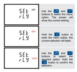
Hold the *MA* button for 3 seconds to exit the set up menu.
