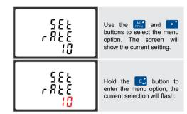
Use the exist and buttons to choose the desired pulse rate. To save the new setting, hold the exist button for 3 seconds until the selection stops flashing.
